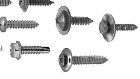
**Teks**<sup>®</sup>: A screw with a drill point that drills its own hole as it is installed. Most Auveco Teks® screws have a #2 point which is recommended for material up to .110" thick. The higher the drill point number, the thicker the material it can drill through. Once the metal is penetrated, the Teks® fastener functions as a conventional tapping screw.
